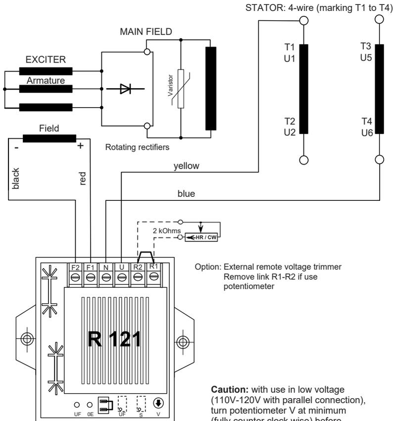
**Caution:** with use in low voltage (110V-120V with parallel connection), turn potentiometer V at minimum (fully counter clock wise) before first power-up.
