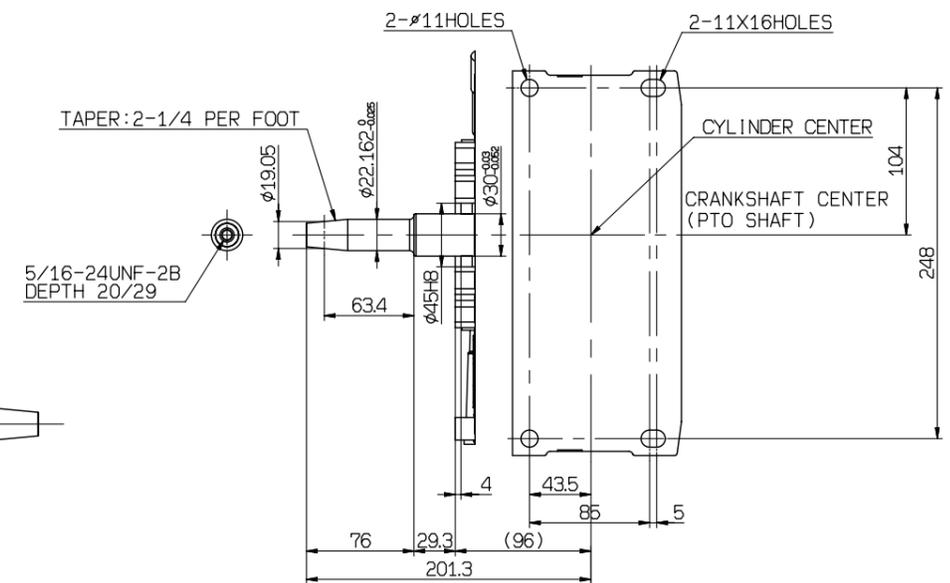
ENGINE MOUNTING PLATE AND PTO SHAFT
