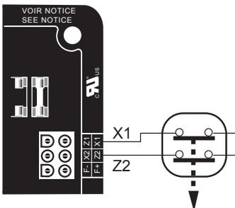
The exciter is switched off by disconnecting the AVR power supply (1 wire on each auxiliary winding) - contact rating 16 A - 250 V A.C.
