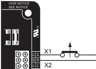
The exciter is switched off by disconnecting the AVR power supply (1 wire - X1 or X2). Contact rating: 16 A - 250 V A.C.
