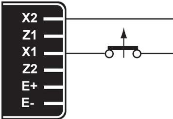
The exciter is switched off by disconnecting the AVR power supply (1 wire - X1 or X2).
