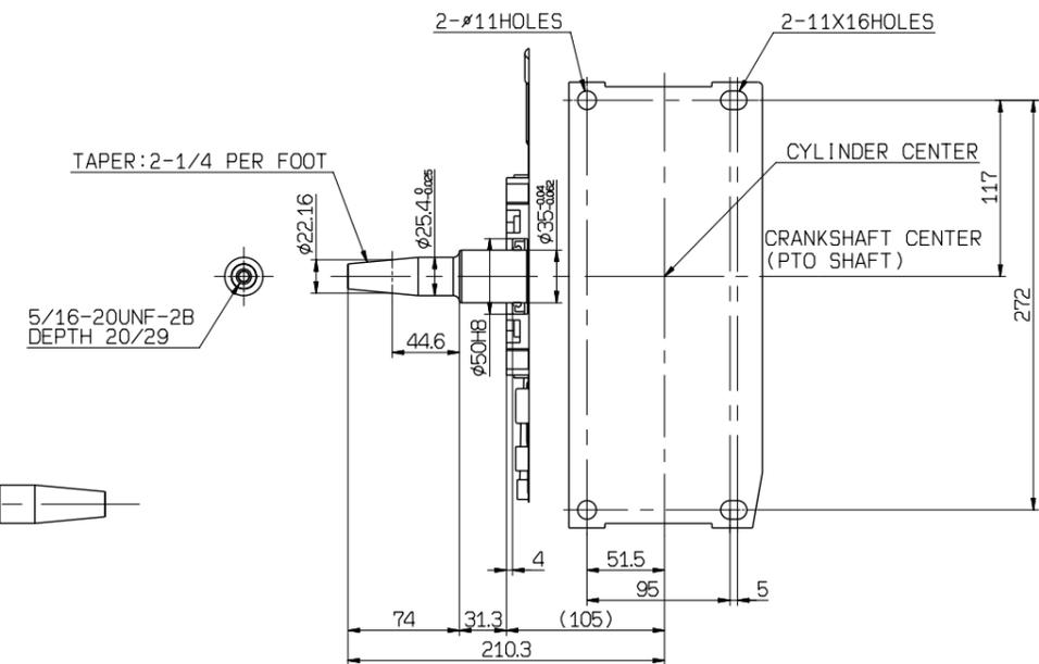
ENGINE MOUNTING PLATE AND PTO SHAFT
