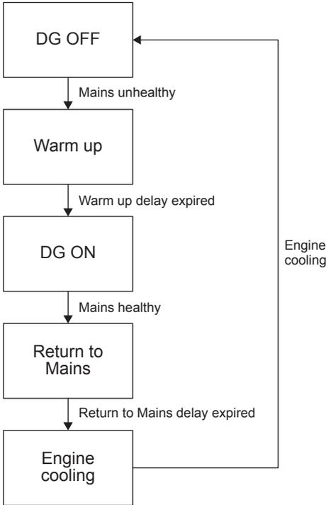
AMF mode is activated when Site monitoring, Cyclic and Exercise modes are disabled, and Mains monitoring is enabled.
