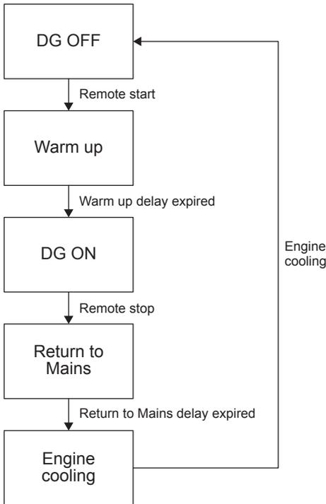
To use the Remote start/stop mode, configure one of the digital input as Remote start/stop (Latched type input) and set the controller to Auto mode. Disable Site monitoring and Cyclic mode.
