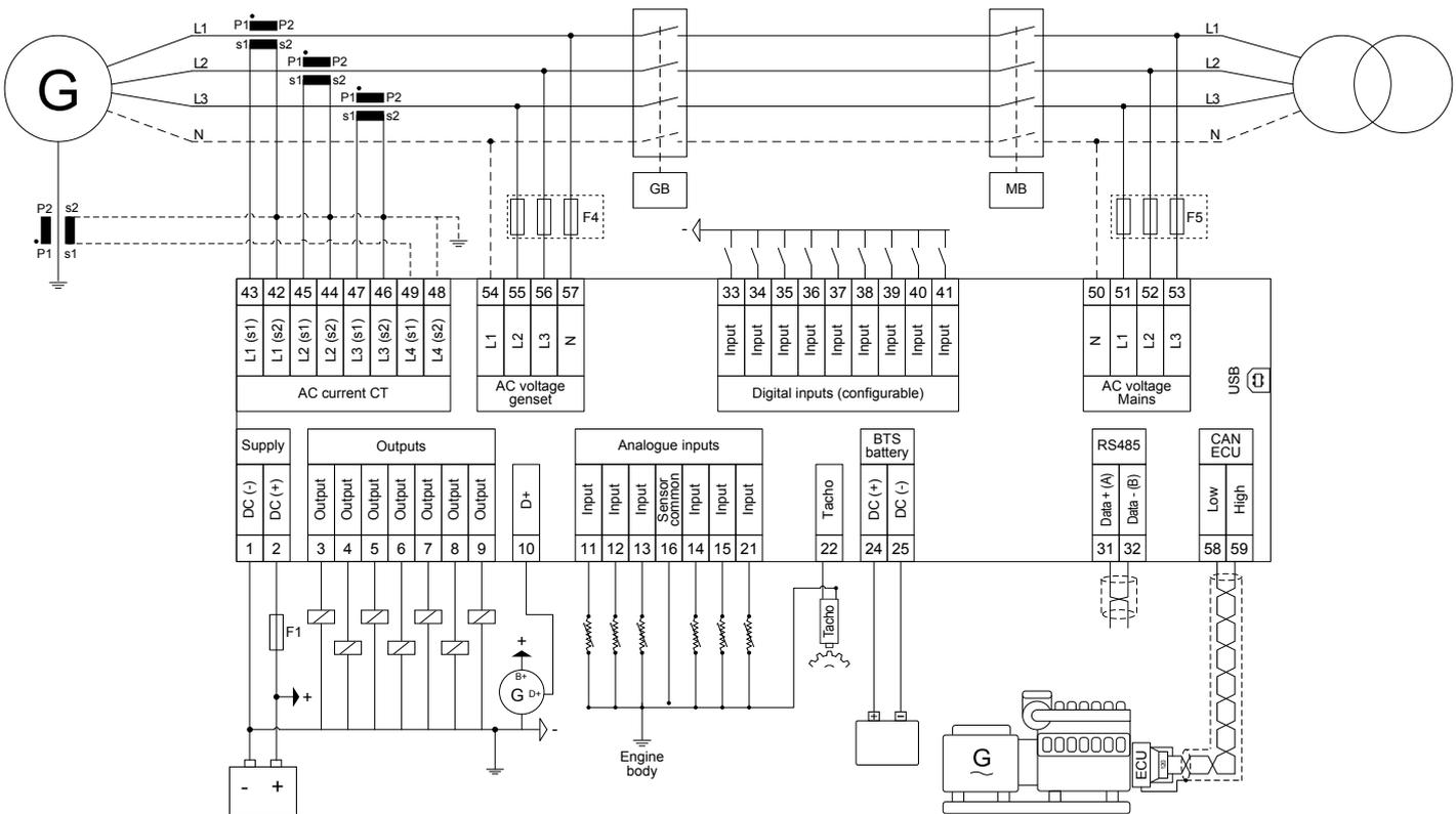
**Figure 4.2** SGC 421 typical wiring
