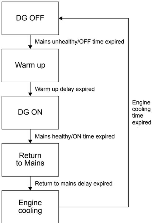
Cyclic mode is used to run the genset for a pre-specified time for a maximum cycle of 12 hours. The genset running time is configurable.
