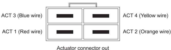
It is recommended to follow the connection details of the Rotary actuator connector and SGC 121.
