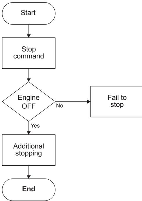
When the controller receives the Stop command, it goes to the Stop state, starts the Stop action time and activates the Stop solenoid output.
