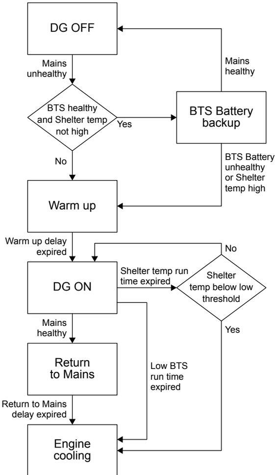
Site Battery Monitoring mode enables the controller to monitor the health of the Site battery and Shelter temperature. The controller manages the power sources (mains/genset) to keep the battery charge within the specified threshold.
