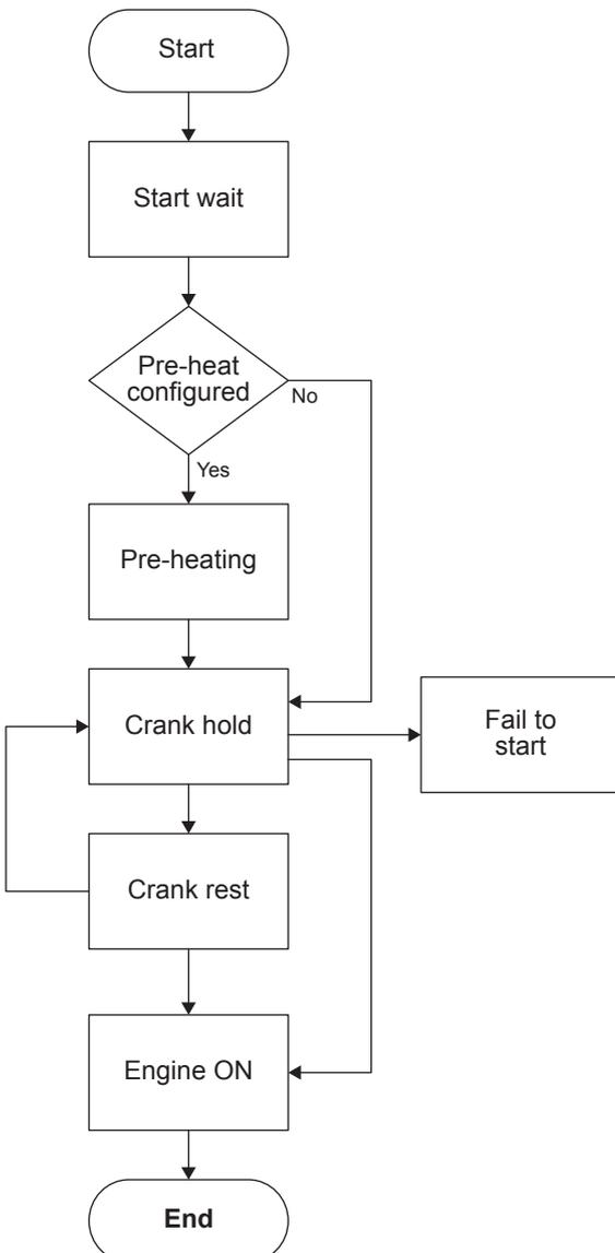
When the controller receives the Start command, it goes to the Start wait state.
