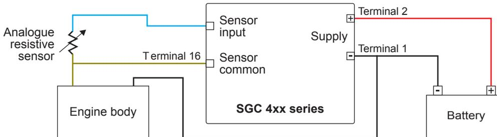
\*SCP connections for Analogue input 2 used as *Fuel level sensor* with the reference configured as *Battery Negative*
